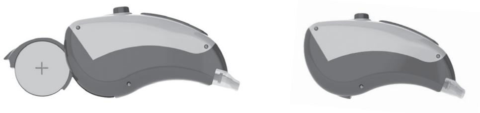
**TIP:** When your device is not in use, make sure you open the Battery Compartment Door to avoid draining your battery's power so it lasts longer.
